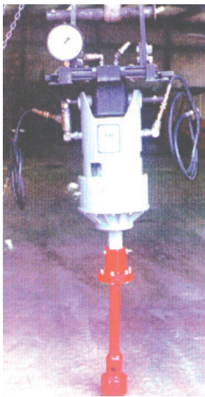
Figure 9.10 Differential Pressure Torque Indicator
