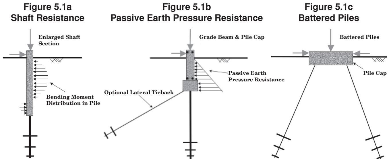
Lateral resistance can also be provided by *passive earth pressure* against the structural elements of the foundation. The resisting elements of the structure include the pile cap, grade beams, and stem walls. The passive earth pressure against the structural elements can be calculated using the Rankine method.
