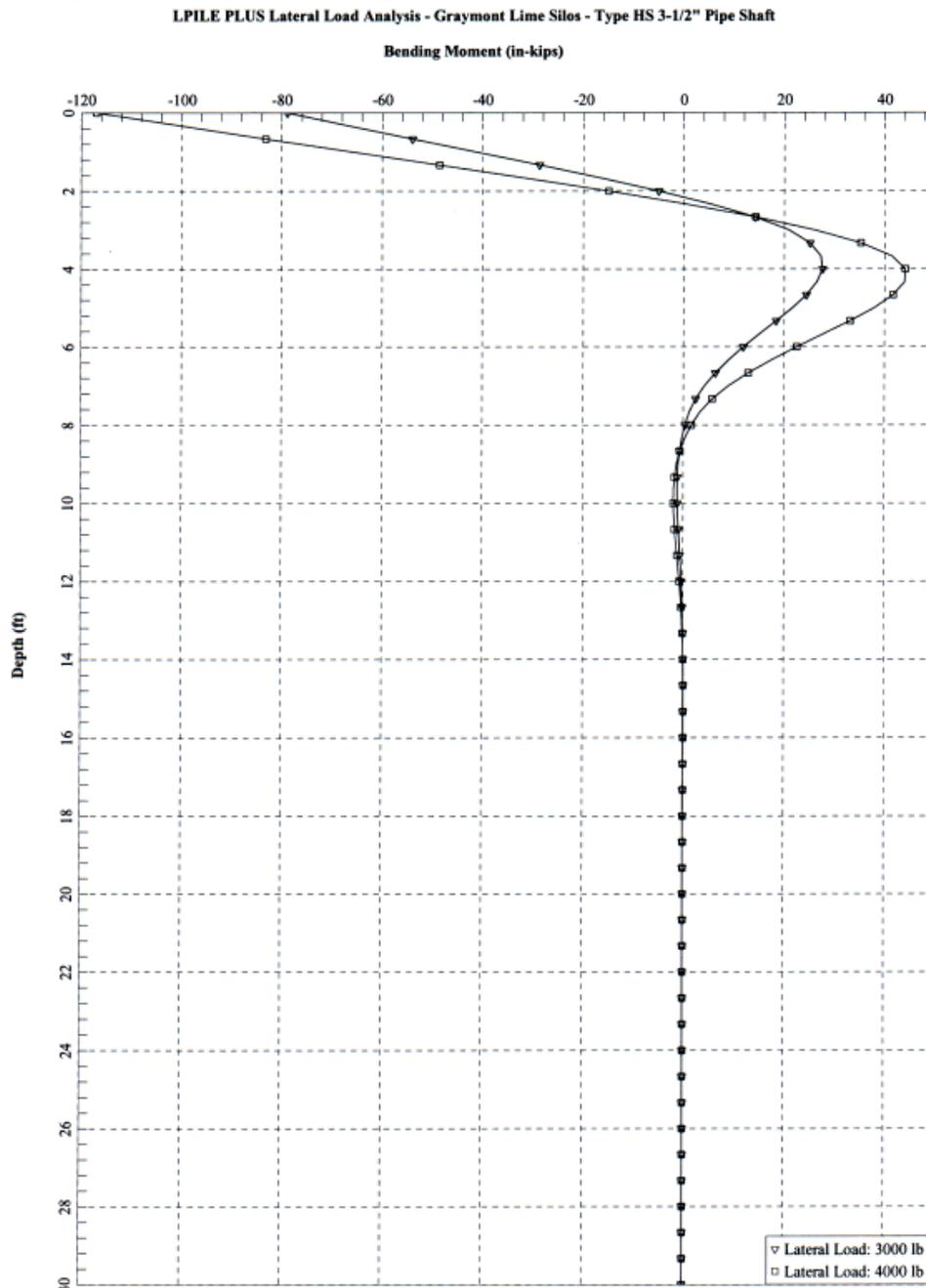
Many geotechnical consultants use LPILE<sup>PLUS</sup> or other soil-structure-interaction programs to predict soil-pile response to lateral loads.
