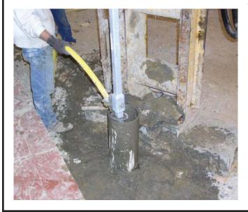
**Pre-Production Performance Test:** A full-scale load test meeting ASTM D1143, Standard Test Method for Piles Under Static Axial Compressive Load, was performed on the test pile. At the maximum compression load of 80 tons and after being held for a 12-hour interval, total deflection was 0.9 inches. After the load was completely removed, net deflection (after rebound) was 0.6 inches. This performance was sufficient to start the installation of the production piles.
