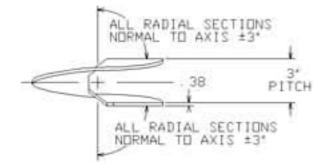
HELIX MUST BE FORMED BY MATCHING METAL DIE (SIDE VIEW OF TRUE HELICAL FORM)
