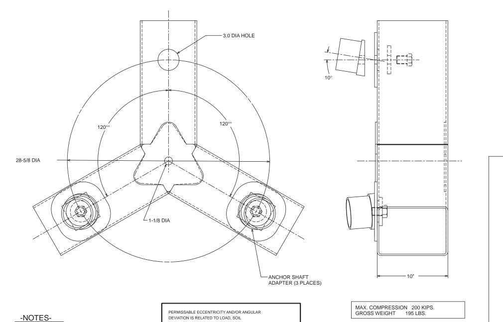
1. HOT DIP GALV. 2. SHIPPED UNASSEMBLED. DEVIATION IS RELATED TO LOAD, SOIL
